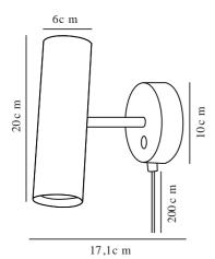
Voltage (V): 230 Volt IP degree: IP20
