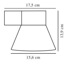
Voltage (V): 220-240 Volt IP degree: IP54 Maximum bulb wattage (W): 25 Class (Class 1, Class 2, Class 3): Class 1 (Earth contact) Socket type: GU10 Parallel connection: True
