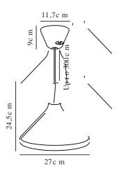
Voltage (V): 230 Volt IP degree: IP20 Maximum bulb wattage (W): 60W Class (Class 1, Class 2, Class 3): Class 2 (Double isolated) Socket type: E27 Dimmerable: Yes with compatible bulb
