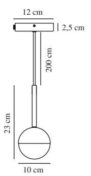
Voltage (V): 230 Volt IP degree: IP20 Maximum bulb wattage (W): 5W Class (Class 1, Class 2, Class 3): Class 2 (Double isolated) Socket type: G9
