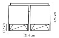
Voltage (V): 230 Volt IP degree: IP20 Maximum bulb wattage (W): 2x50W
