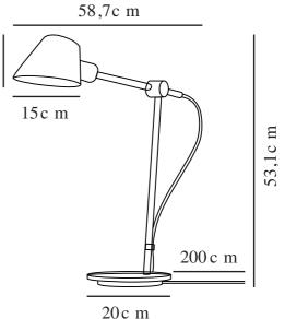
Voltage (V): 230 Volt IP degree: IP20 Maximum bulb wattage (W): 60W Class (Class 1, Class 2, Class 3): Class 2 (Double isolated) Socket type: E27 Switch placement: On the fixture
