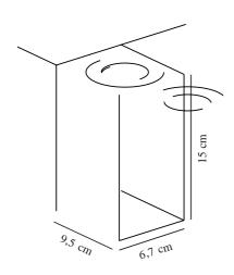
Voltage (V): 230 Volt IP degree: IP44 Class (Class 1, Class 2, Class 3): Class 1 (Earth contact) Socket type: LED Module
