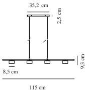
Voltage (V): 220-240 Volt IP degree: IP20 Class (Class 1, Class 2, Class 3): Class 2 (Double isolated) Socket type: LED Module
